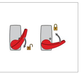
In the event of maintenance, malfunctioning or emergency, pull the lock release lever VALSB down and turn it to the right or lower the lock release lever LOKSBM (if installed) and move the door wings manually into the open position.
