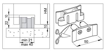
The measurements of the code 0KP369 floor guide for glass door wings are indicated in the diagram.
