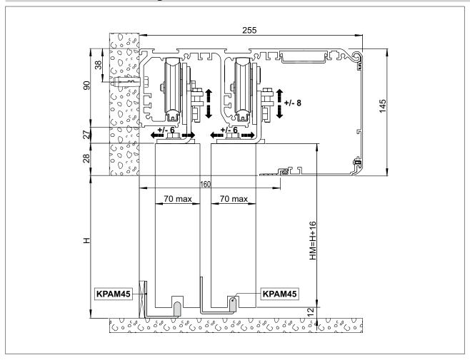
The VALOR TR automation wall fixing measurements are illustrated in the diagram, considering that the door wing profiles are not of our production.
