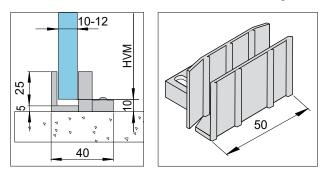
The measurements of the code KPAM35 floor guide for telescopic door wings are indicated in the diagram.
